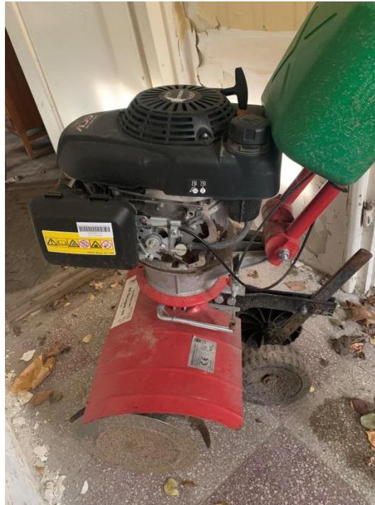
Figure 5.18 Rotary hoe (E. Takács)
