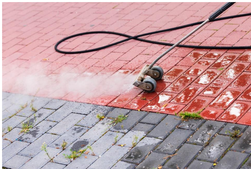
Figure 5.15 Weed killing steamer ( https://www.shutterstock.com )
